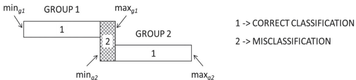
Figure 3. Procedure for selecting appropriate acoustic features. The value of 1 indicates correct classification, and the value of 2 indicates incorrect classification. Parameters " \max_{g1} " and " \min_{g2} " indicate maximum and minimum threshold limits for incorrect classification.
