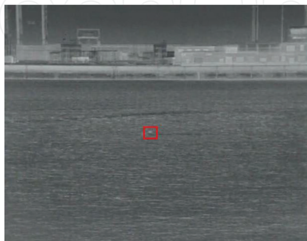
Figure 17. Drifting mine in the Zeebrugge harbour as captured by the MicroCompass MWIR sensor on the P901 Castor.
