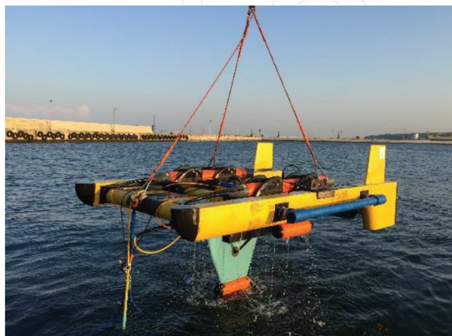
Figure 10. The gradiometer was attached to a platform with remotely controlled depth/altitude. The system was towed behind a boat. This picture was taken by TNO.
