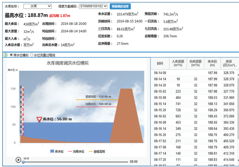
Figure 10. Interface of reservoir regulation.
