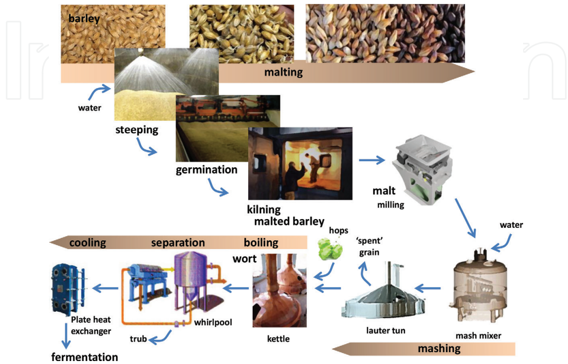
Figure 1. Malting and brewing process. First steps mashing and wort preparation.
