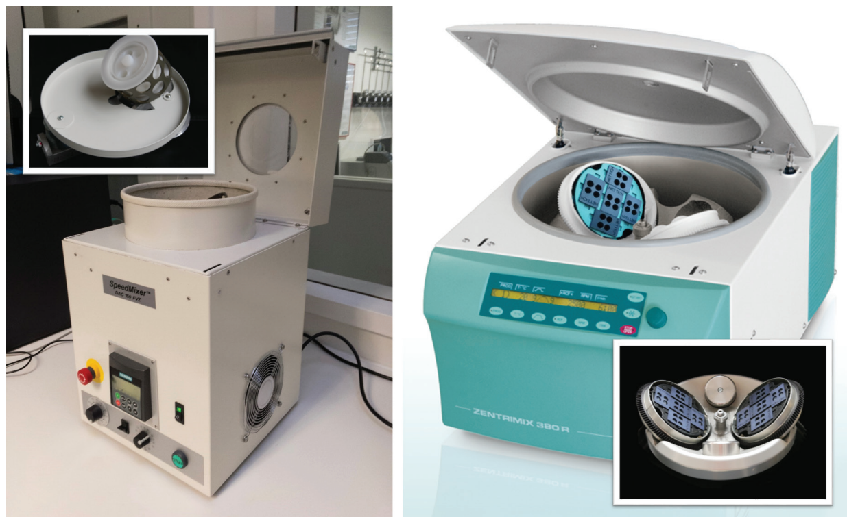
Figure 8. Pictures of the two dual centrifuges: the Speedmixer DAC 150 FVZ (left) and the ZentriMix 380 R (right). Their respective rotors with typical vial holders are shown in the small pictures.
