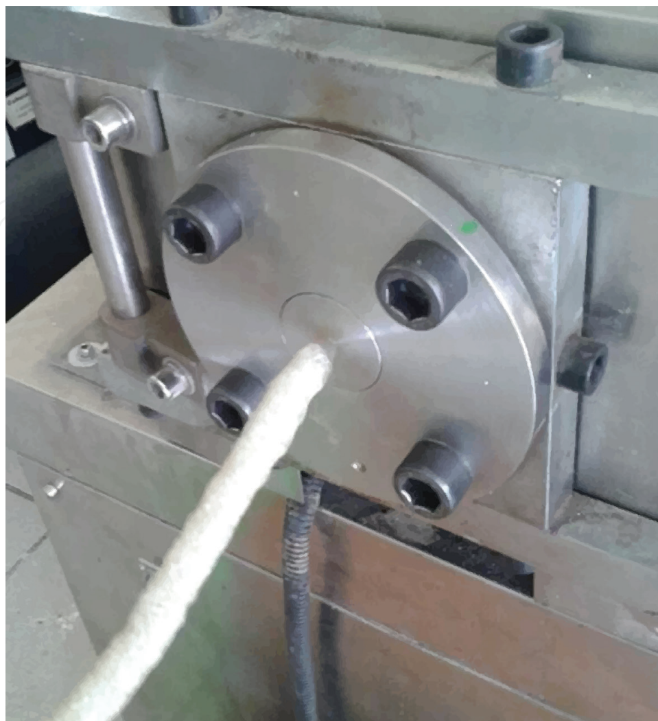
Figure 1. Expansion of cornstarch due to extrusion.
