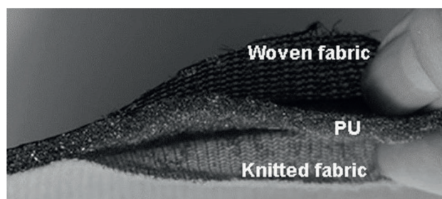
Figure 3. Composite material for car seat upholstery.
