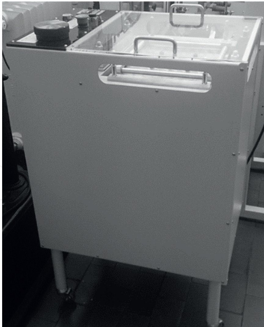
Figure 12. The device for measuring uniaxial and biaxial cyclic stress.
