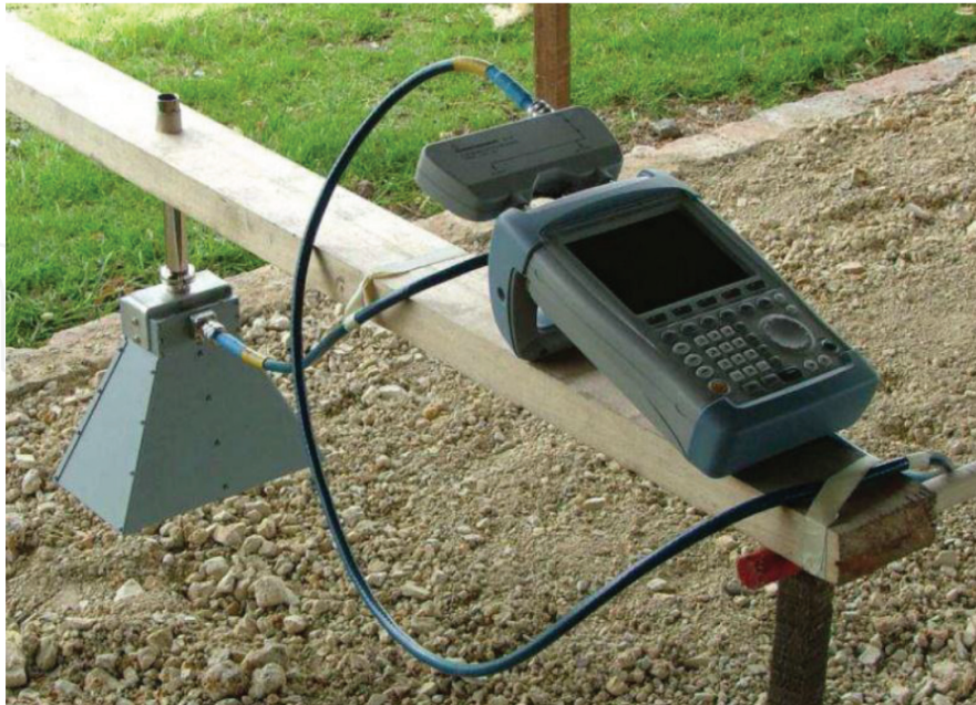
Figure 12. The UWB SFCW GPR system emulated using the hand-held VNA connected to the horn antenna via a 50-Ohm N-type coaxial cable.
