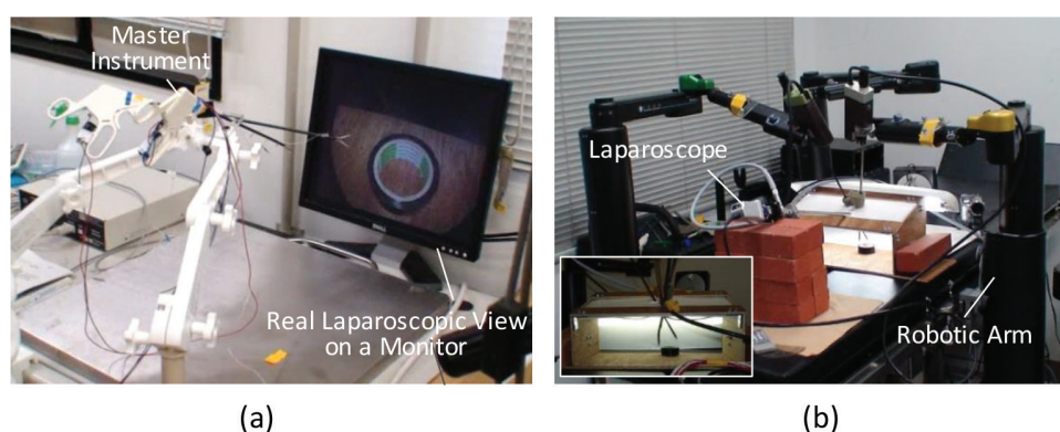
Figure 5. Object-touching task during the task in iSPS: (a) master set-up and (b) slave set-up.
