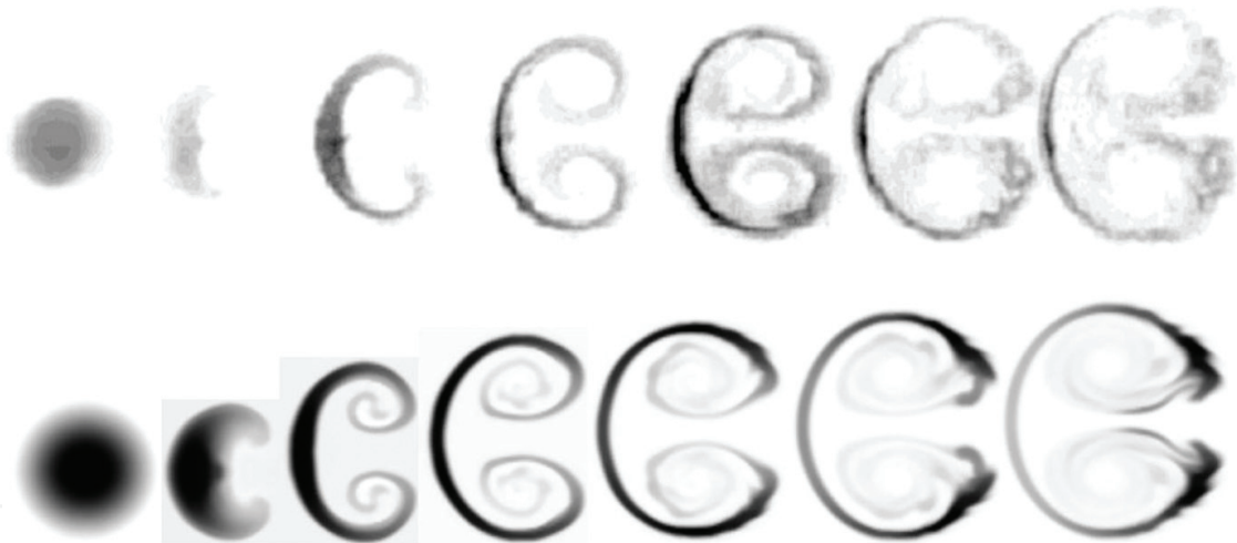
Figure 9. Evolutions of \text{SF}_6 gas cylinder, upper row corresponding to experiment, lower row corresponding to numerical simulation by MVFT program, the time sequences are 0, 50, 190, 330, 470, 610, and 750 \mu\text{s} severally.
