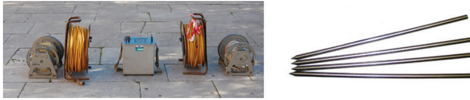
Figure 2. Resistivity equipment: left, automated resistivity metre and cables; right, stainless steel electrodes.
