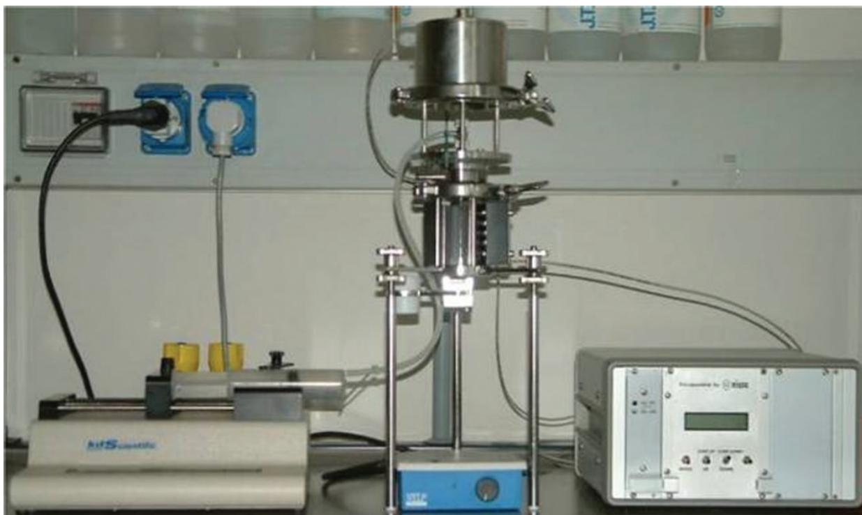
**Figure 1.** Prilling apparatus (Nisco Inc.) at the Department of Pharmacy, University of Salerno.
