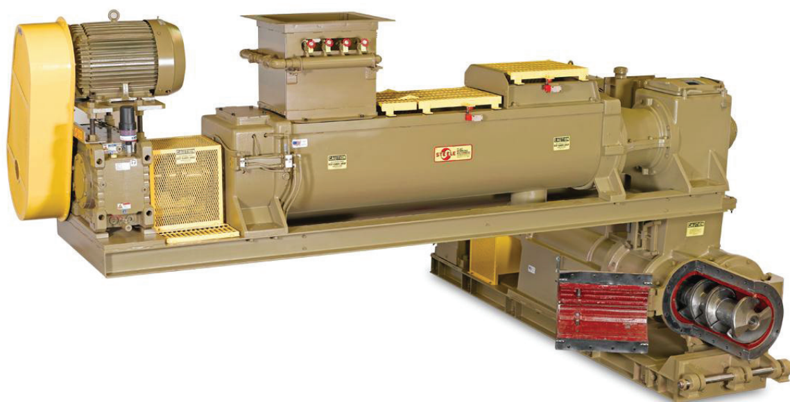
Figure 1. General view of the extruder (bottom) and pug sealer.
