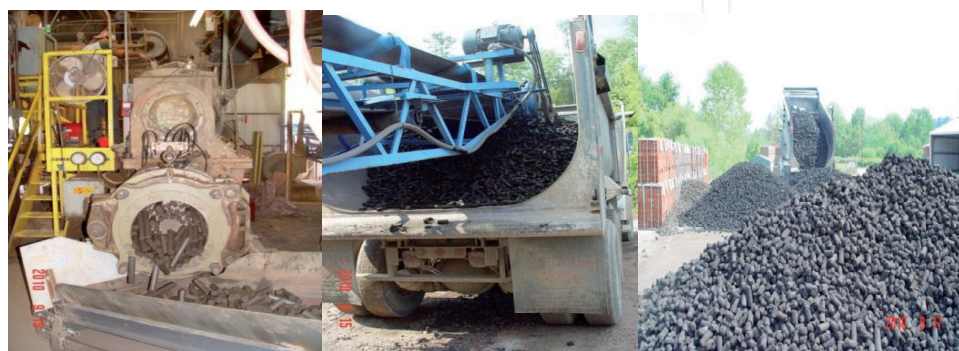
Figure 9. Production (at left), loading (in the middle), and stockpiling of the green BREX for ferroalloy production.
