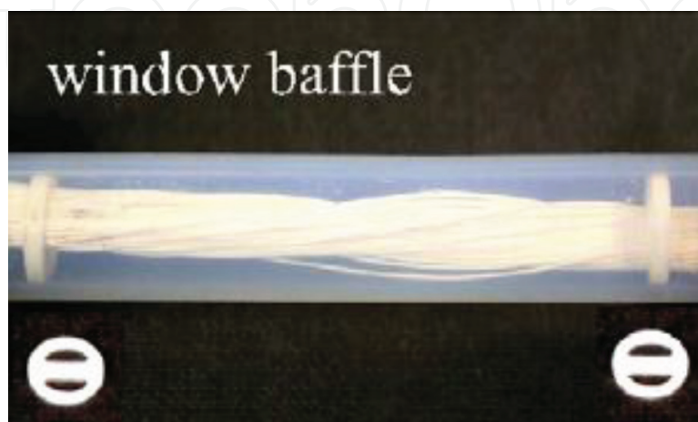
Figure 9. Hollow fiber module with window baffles [38].
