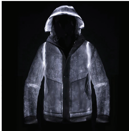
Figure 13. LED jacket, fabric woven from optical fibers within nylon and steel fabric [39].
