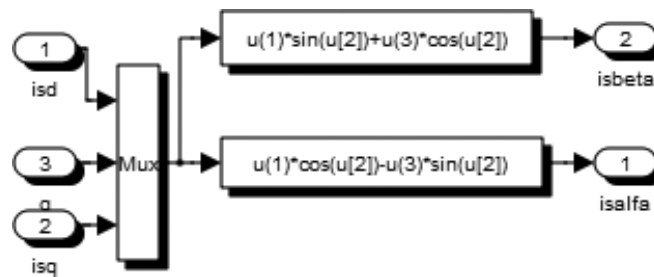
Figure 24. The Simulink implementation of the reverse Park transformation.
