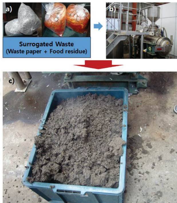
Figure 2. Biochar products process from waste by hydrothermal carbonization; (a) surrogated municipal solid waste, (b) pilot-scale hydrothermal treatment systems, and (c) biochar products.
