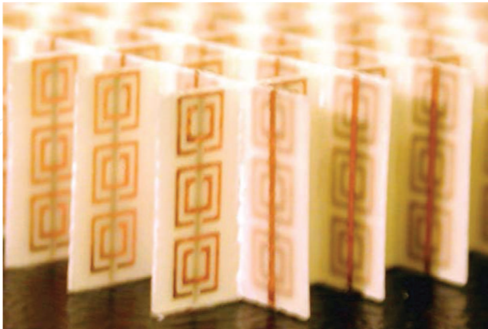
Figure 1. Optical image of a classical metamaterial structure that operates at a resonant frequency of 10.5 GHz[8] (Reproduced with permission of American Association for the Advancement of Science via Copyright Clearance Center).
