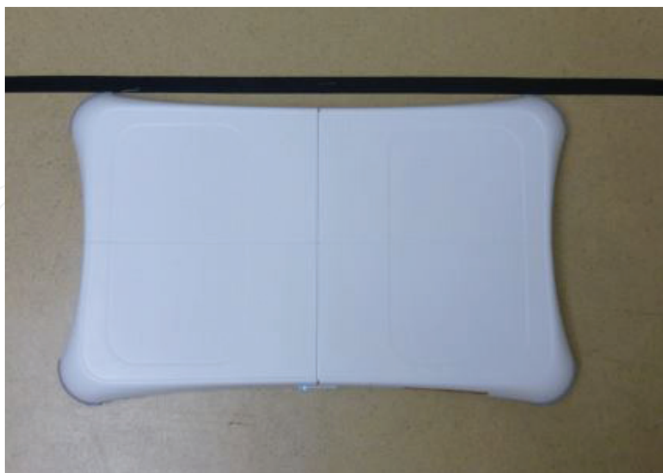
Figure 7. Recently, the Wii Balance Board has been much used in the field of medical research, and it has been reported that results from the Wii Balance Board correlate closely with those of commercially available force plates.
