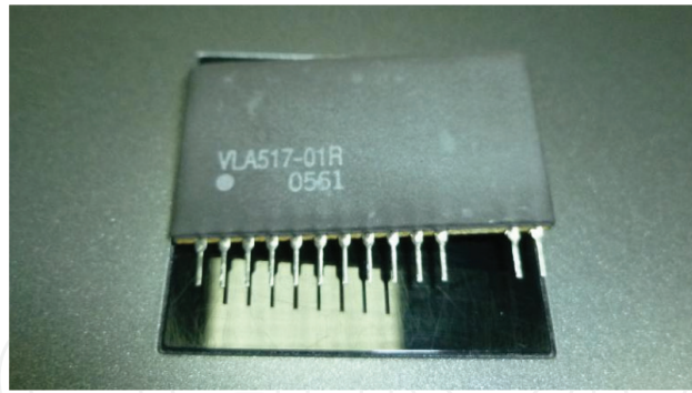
Figure 17. Hybrid integrated circuit, type VLA 517–01R–FUJI, driver [14].
