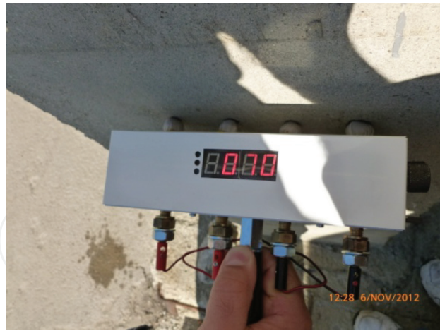
Figure 8. The measurement of a concrete pillar, first measurement.
