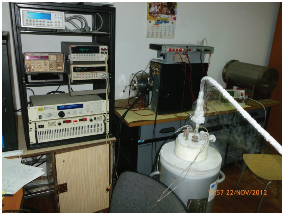
Figure 30. The experimental setup of the quench protection system of the superconducting coil during the experiments (the superconducting coil and the power supply are connected) [14].
