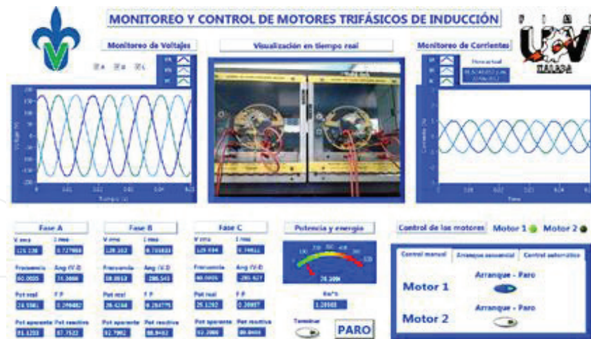
Figure 4. Front panel of the main virtual instrument developed for the control of two AC induction motors [17].
