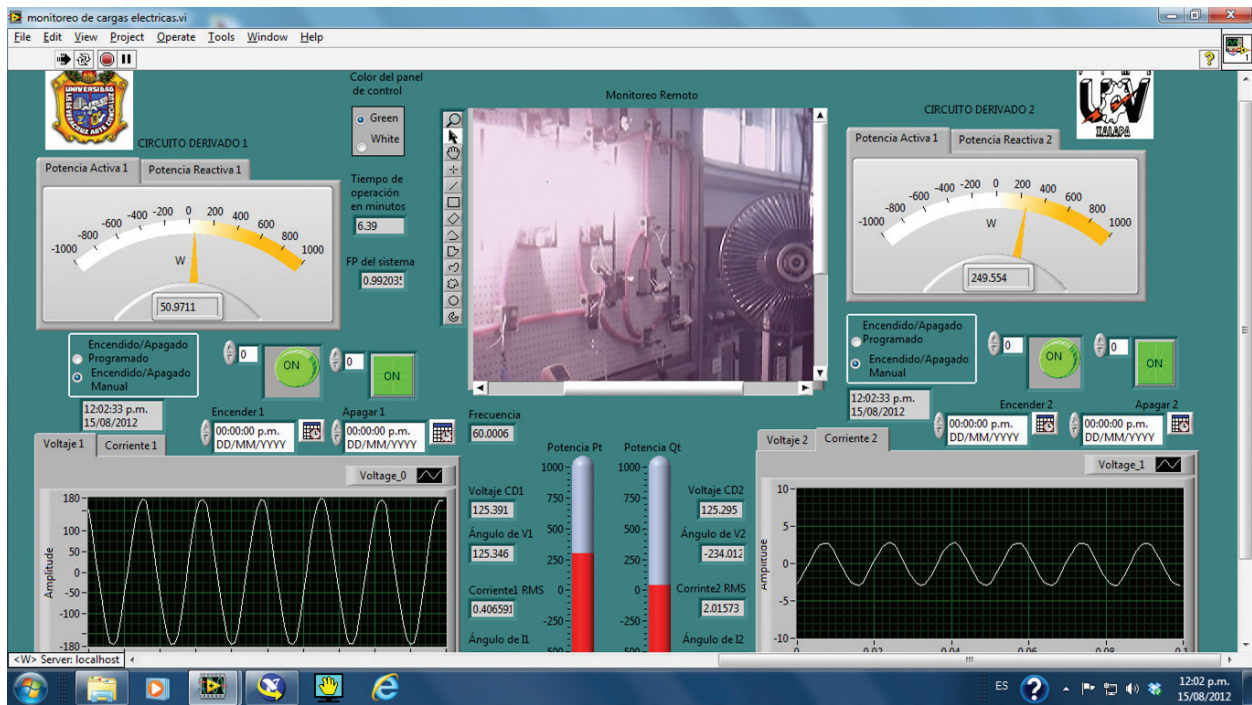
Figure 5. Front panel of the virtual instrument for the control and monitoring of residential electrical circuits [18].
