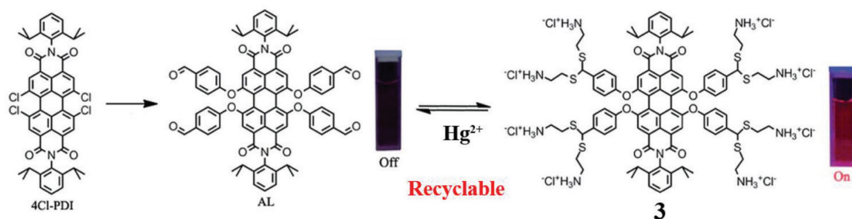
Figure 3. Synthesis approach and sensing mechanism of chemsensor 3.
