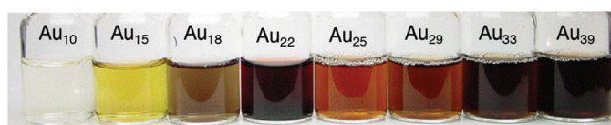
Figure 2. Photograph of aqueous solutions of glutathionate-protected Au n clusters [3].
