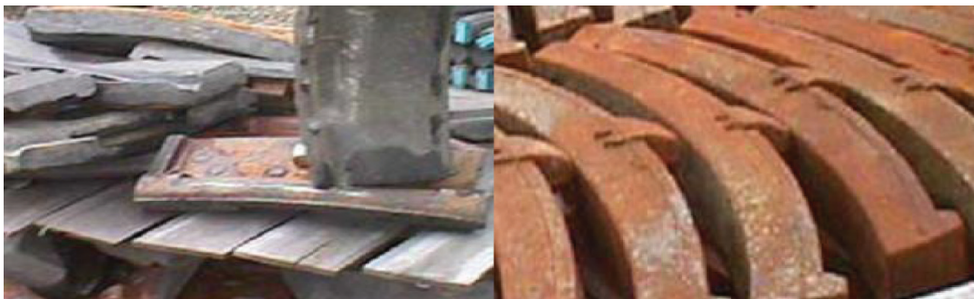
Figure 2. The cast brake shoes with wear indicators.
