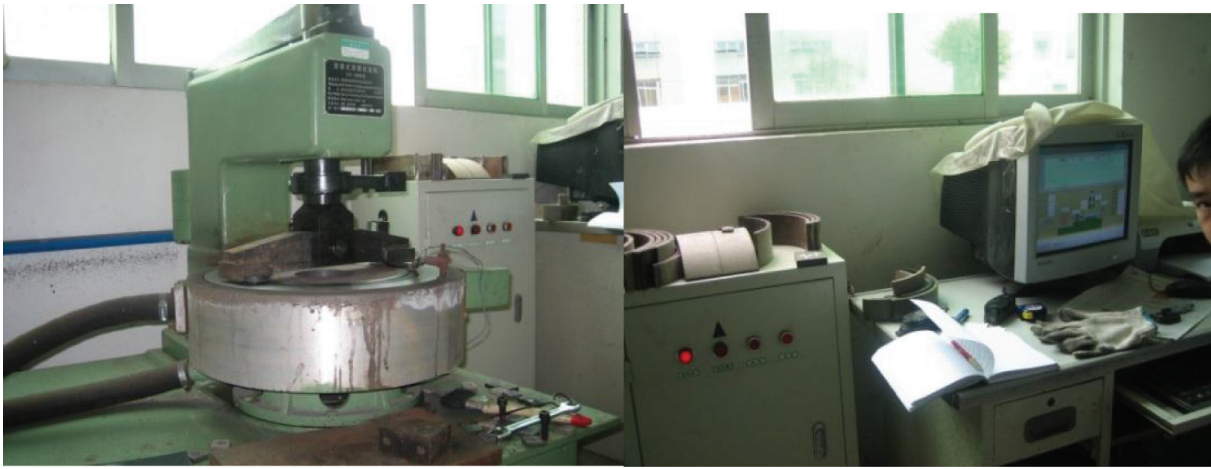
Figure 12. X-MSM constant speed friction material tester and monitor/control unit.
