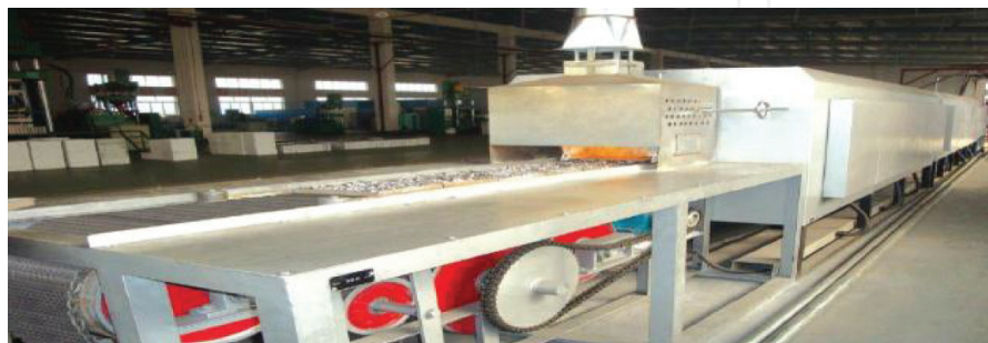
Figure 10. Mesh belt continuous resistance furnaces.
