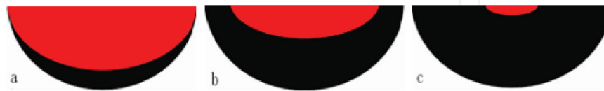
Figure 14. Schematic diagram of the solidification process of silicon cake: (a) the initial stage, (b) the intermediate stage and (c) the end stage.
