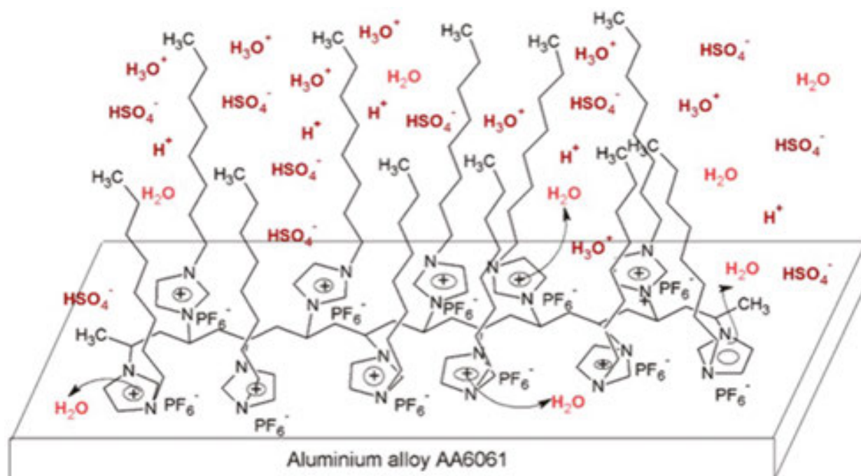
Figure 6. Schematic model of the corrosion protective action of poly(1-vinyl-3-alkyl-imidazolium Hexafluorophosphate toward AA 6061, proposed in [46].
