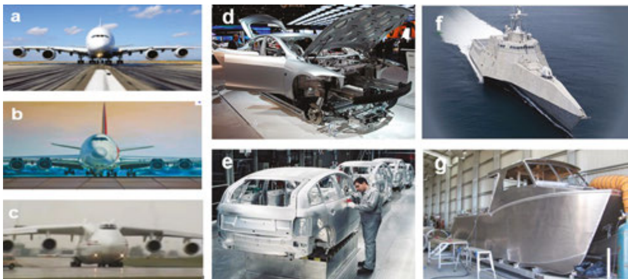
Figure 1. Various kinds of vehicles composed by aluminum alloys. (a) Airbus A380 [8], (b) Boeing 747 [9], (c) Antonov 225 [10], (d, e) aluminum car bodies [11], (f) aluminum ship type Littoral Combat Ships [12], (g) aluminum sport boat [13].
