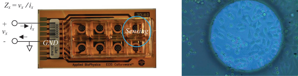
Figure 2. The 8E10W system. Each system has 8 separated wells for cell culture and 10 electrodes of 250 \mu\text{m} diameter by well ( www.biophysics.com ). On the right side, an electrode with the Chinese hamster ovary fibroblast cell line, AA8 (American Type Culture Collection), cultured over the surface of one circular electrode can be seen.
