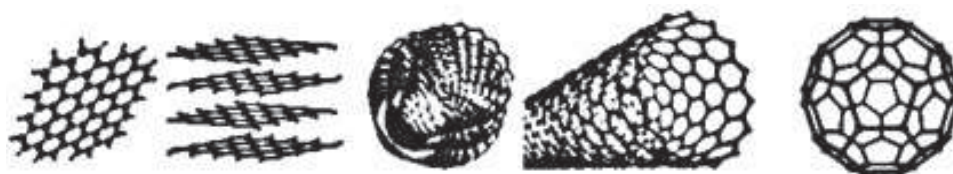
Figure 1. Structure of allotropes of carbon: (a) Graphene; (b) Graphite; (c) MWCNT; (d) SWCNT; (e) Fullerene.
