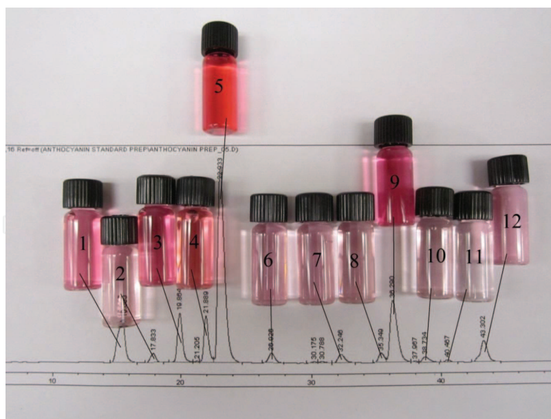
Figure 4. Preparative HPLC chromatogram showing separation of anthocyanin monoglucosides and acyl-glucosides of Cabernet Sauvignon grapes from Washington State (USA). Anthocyanin fractions are shown approximately above of each major peak and were collected directly from the elutant at pH ~ 1.8. Peak assignment: (1) delphinidin-3- O -glucoside, (2) cyanidin-3- O -glucoside, (3) petunidin-3- O -glucoside, (4) peonidin-3- O -glucoside, (5) malvidin-3- O -glucoside, (6) delphinidin-3- O -acetyl-glucoside, (7) petunidin-3- O -acetyl-glucoside, (8) peonidin-3- O -acetyl-glucoside, (9) malvidin-3- O -acetyl-glucoside, (10) malvidin-3-(6- O -caffeoyl)-glucoside, (11) petunidin-3-(6- O -coumaroyl)-glucoside, (12) peonidin-3-(6- O -coumaroyl)-glucoside (shoulder), and malvidin-3-(6- O -coumaroyl)-glucoside.
