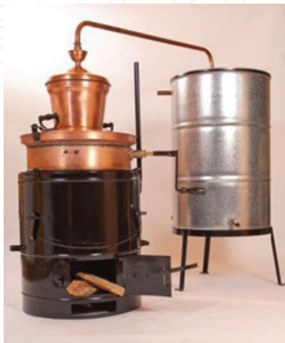
Figure 3. Traditional copper alembic pot still. The hat plays a role in the reflux because the vapour came in and will partially condense and run back down to the original liquid in the boiler and be redistilled. The flavour of final spirits was influenced by the shape and size of the hat [19].
