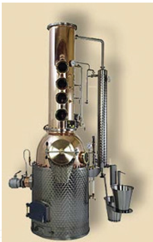
Figure 4. Steam-fired batch distillation column still with three trays and dephlegmator above them. Reflux rate is varied by changing the cooling rate in dephlegmator.
