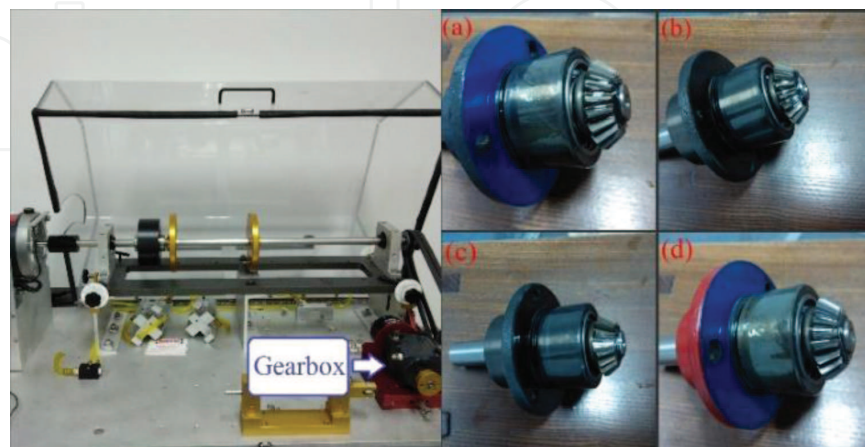
Figure 4. The experiment rig and the four bevel gears with different damages. (a) Normal gear, (b) gear with broken tooth, (c) gear with missing teeth, and (d) gear with worn tooth.
