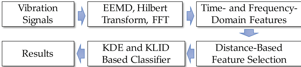
Figure 2. The procedures of the proposed fault diagnosis approach for rotating machinery.
