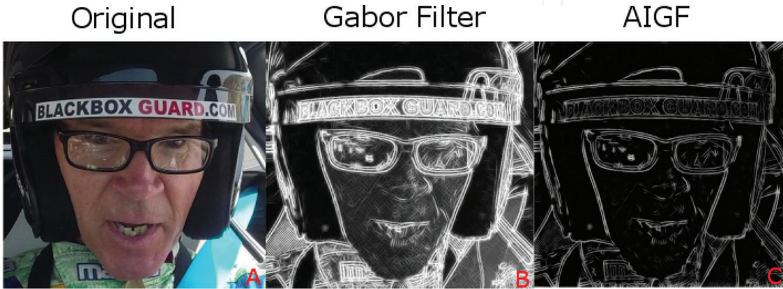
Figure 2. (a) Original frame, (b) result of Gabor energy filter (Eq. (15) with \alpha = 0 ), and (c) result of Anisotropic Gabor Energy Filtering.
