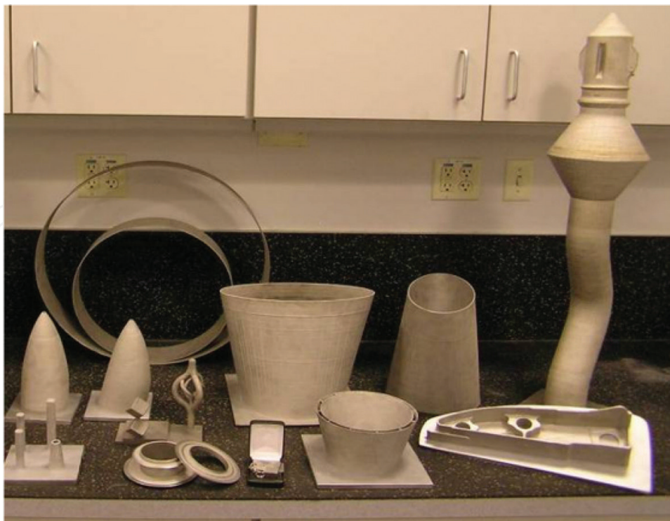
Figure 12. Examples of parts produced by free-form technology [18].
