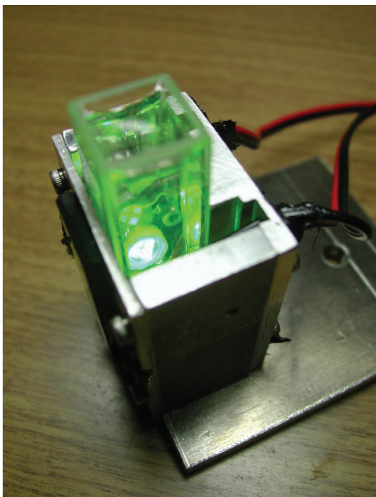
Figure 18. Photograph of excitation by green LED.
