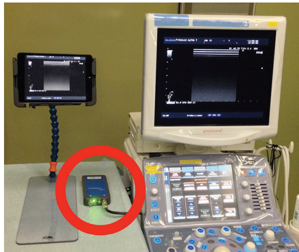
Figure 18. iPad Mini (Apple Japan LLC, Tokyo, Japan), VT-100 wireless video transmitter encircled in red (Scalar Co., Tokyo, Japan), and ProSound Alpha 7 ultrasound equipment (Hitachi-Aloka Medical Ltd., Tokyo, Japan). With our method, ultrasound image signals from the ProSound Alpha 7 are transmitted by a conventional coaxial video cable to the VT-100, then sent wirelessly to the iPad Mini by Wi-Fi without any image reproduction delay.
