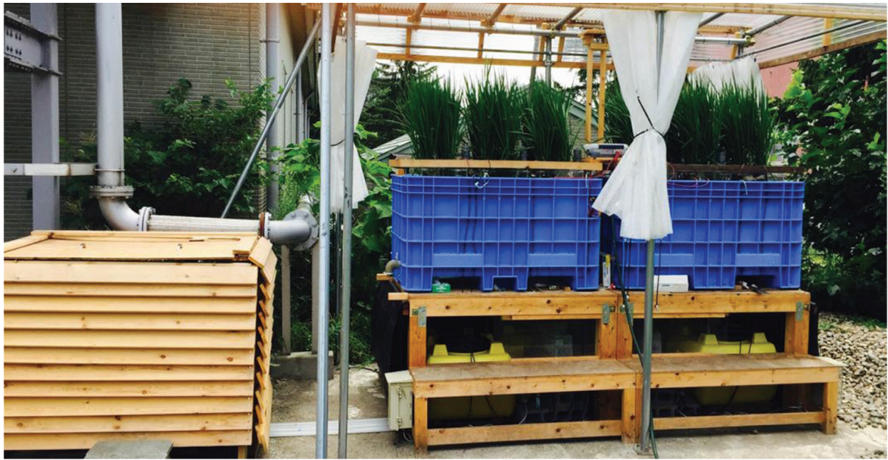
Figure 2. Bench-scale experiment to reveal the performance of treated wastewater irrigation to cultivate rice for animal feeding.
