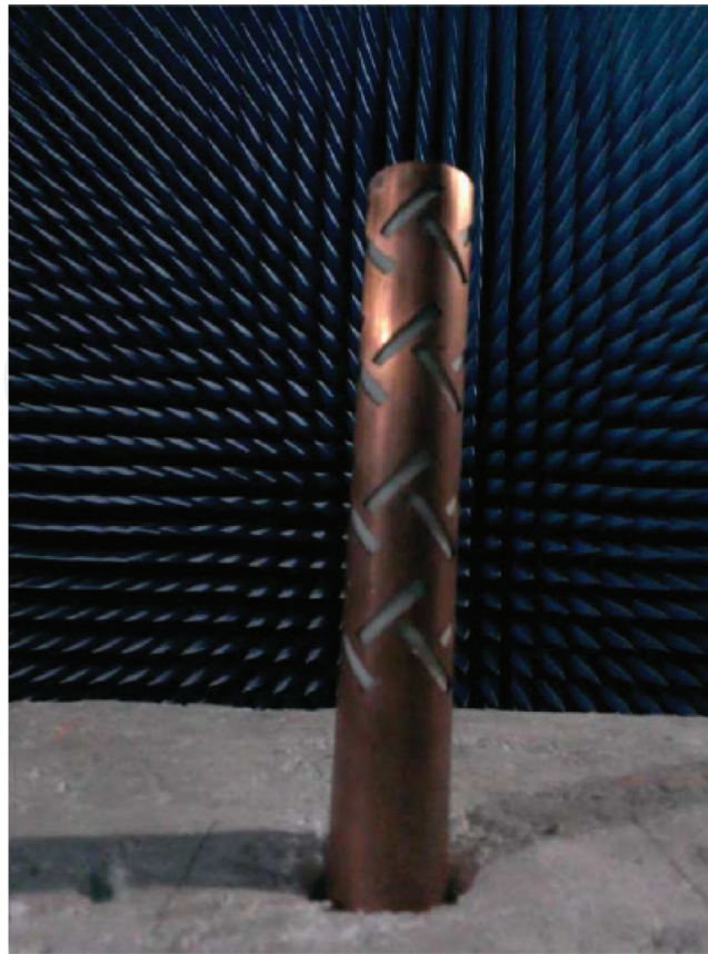
Figure 4. Photograph of the omnidirectional CP antenna being tested in the anechoic chamber.
