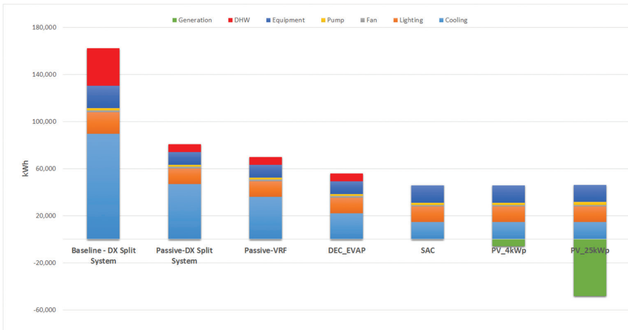
Figure 20. Total annual energy consumption by type using different strategies with renewables (kWh).
