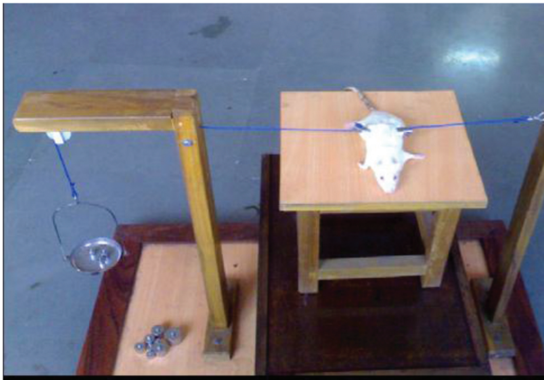
Figure 3. Tensiometer for determination of tensile strength of repaired skin of the albino rat.
