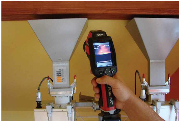
Figure 9. Monitoring the temperature of the wood by thermal imaging can cause distortions to the view of the situation: the areas of high temperature, visible on the screen, can cover layers of much lower temperature, harmless to the larvae (photo by CARSEKT).
