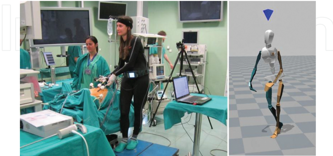
Figure 2. Motion tracking system based on inertial sensors embedded in an elastic suit ( left ). A biomechanical model of the subject is created in real time ( right ).
