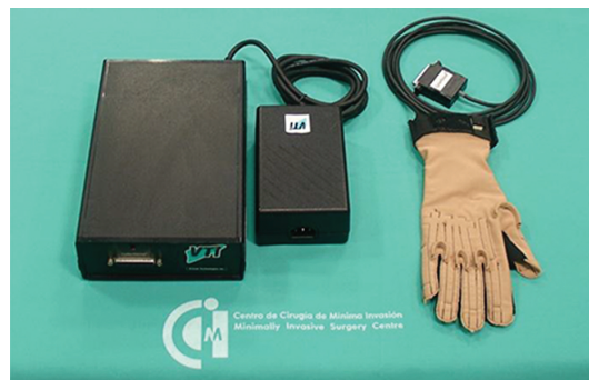
Figure 4. Motion capture data glove CyberGlove® (CyberGlove Systems, San José, CA, USA). This device consists of a series of conductive sensors with resistance flows sensitive to flexion variations.
