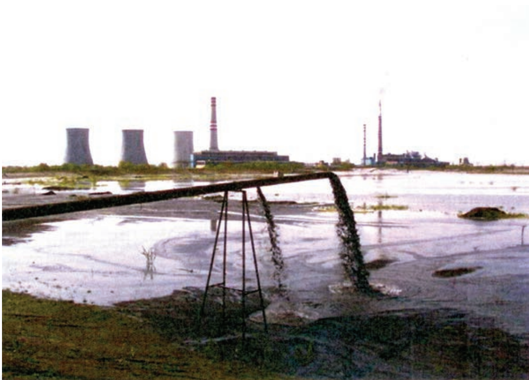
Figure 4. Filling tailing pond.
