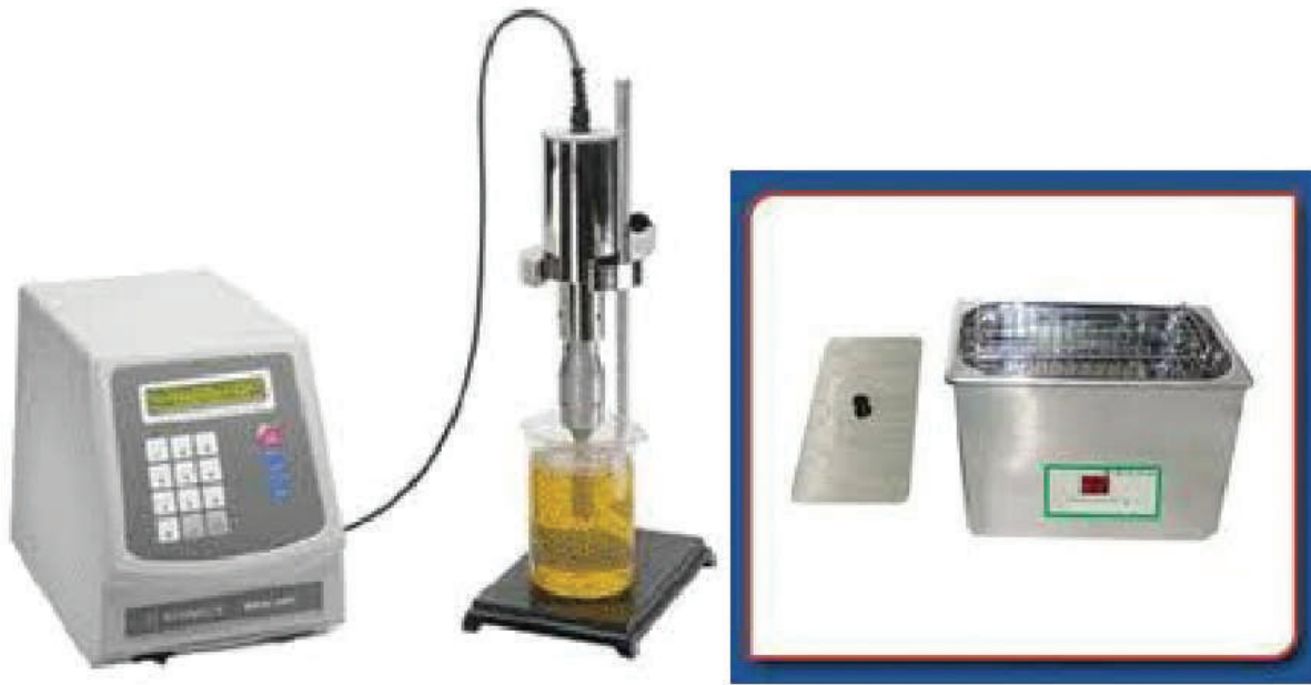
Figure 4. Probe (VCX 500, 20 kHz, 500 W) (left) and bath (POWERSONIC, UB-405, 40 KHz, 350 W) (right) ultrasonic, respectively.
