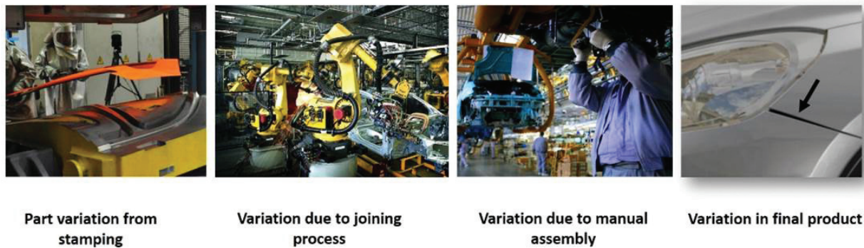
Figure 1. A nonparallel split line, caused by variation due to the stamping, joining and assembly processes.
