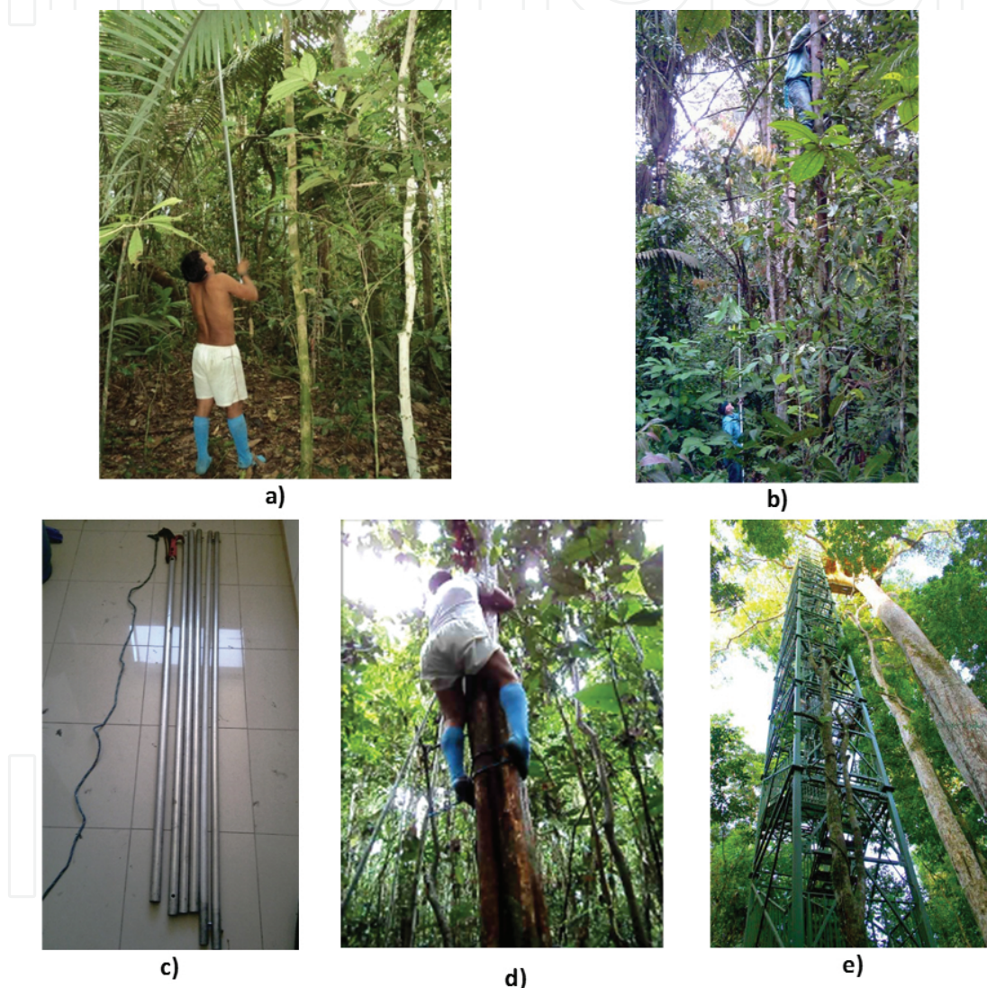
Figure 3. Photographs of leaf sampling process. (a) Collecting leaves using the telescopic pruner (b) climbing trees (c) telescopic pruner 9 m long (d) climbing trees techniques and (e) canopy towers in the study area.
