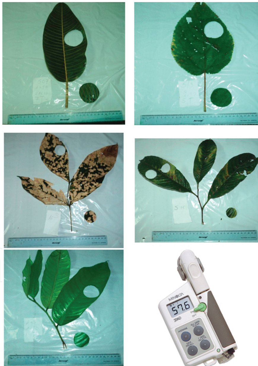
Figure 4. Leaf samples and clipped disks from plants of different species and health status. The last photo shows the SPAD-502 meter.
