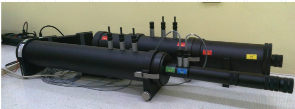
Figure 6. The Kundt device for acoustic measurements.
