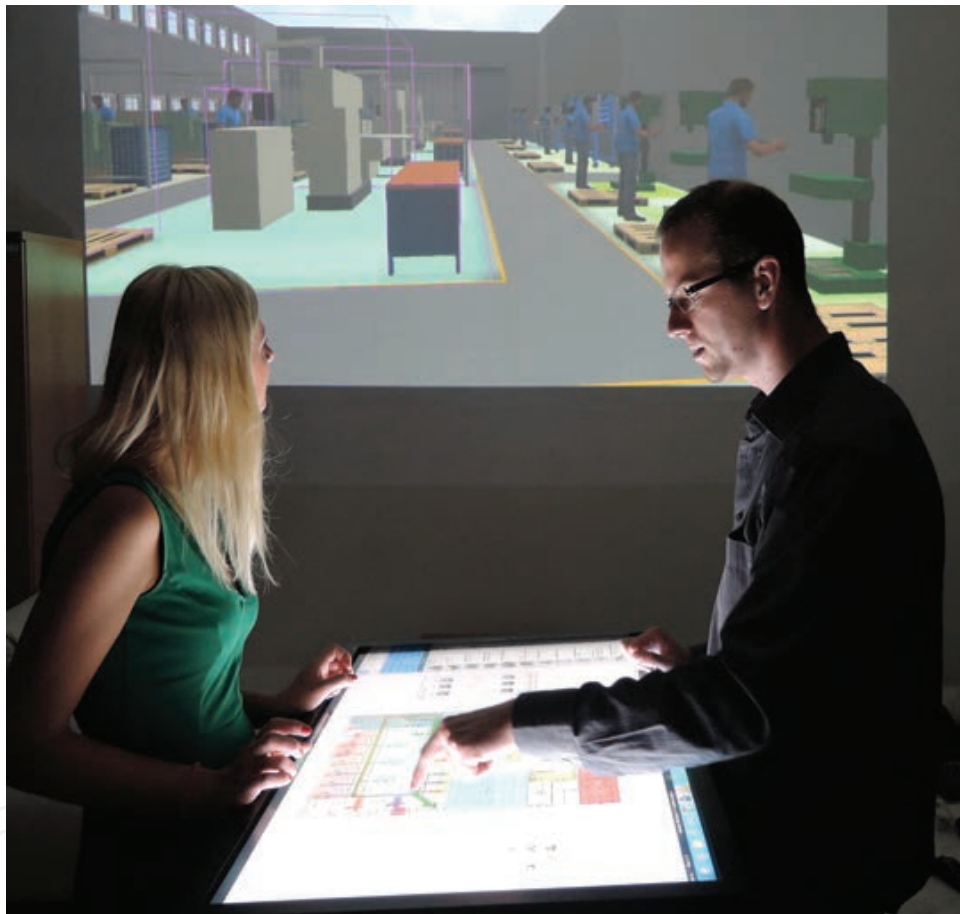
Figure 1. Augmented reality projection table. Touchscreen with black and white 'markers' is shot by a webcam. The marker-based 3D environment is generated and sent to a projector (original solution by Department of Industrial Engineering and Management, University of West Bohemia).
