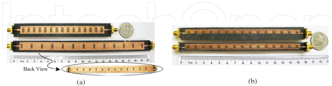
Figure 7. Fabricated LWAs, (a) SIW configuration and (b) HMSIW configuration [7].
