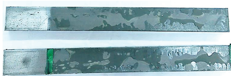
Figure 9. Failure surfaces for the DCB specimen.
