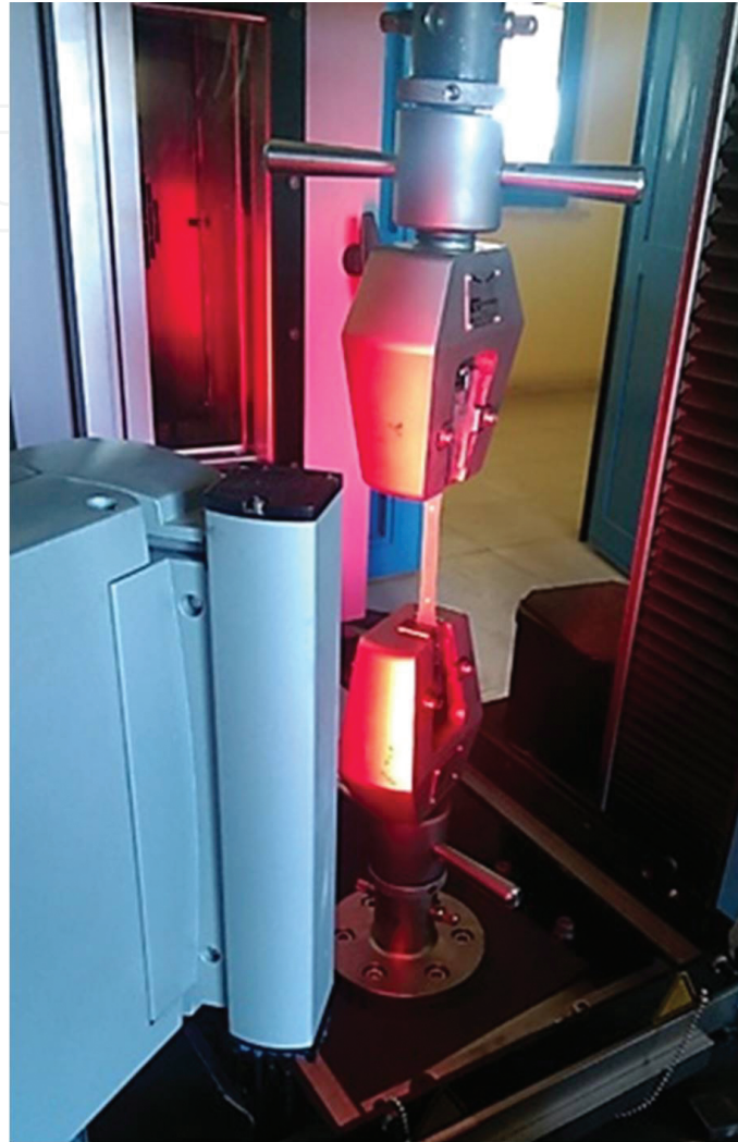
Figure 4. Tensile tester with video extensometer.
