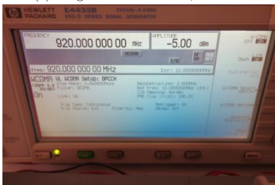
(c) RF generator: 920 MHz, -5 dBm
