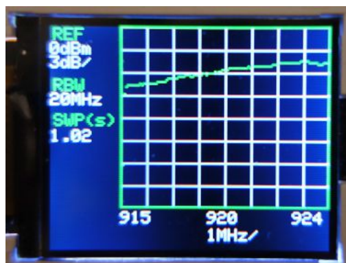
(c) RF in 920 MHz, -5 dBm; RBW 20 MHz, sweep time 1 seconds
