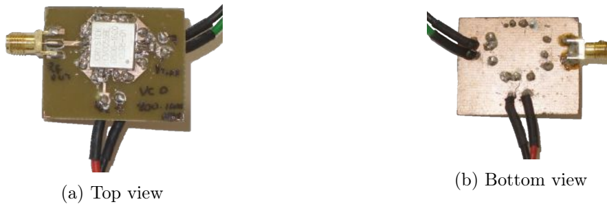
Figure 4.16: VCO CVCO55BE-0800-1600 evaluation board
