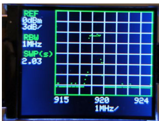
(a) RF in 920 MHz, -5 dBm; RBW 1 MHz, sweep time 2 seconds
